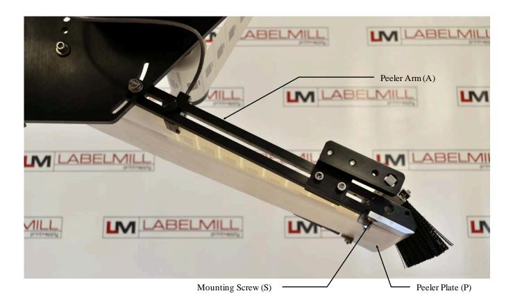
Peeler Plate Adjustment (used to adjust tracking)
