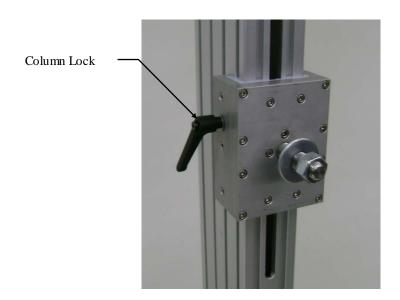
To adjust the T-150 mounting stand, simply loosen the headlocks and adjust to the desired height by turning the column crank. Be sure to lock the headlocks when finished.
