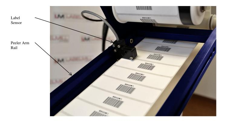
Manual adjustment of the label in relation to the peeler plate is achieved by loosening the thumbscrew on the backside of the label sensor and sliding the assembly up or down on the peeler arm rail.
