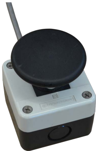
PB-32 Push Button (Remote start trigger)
