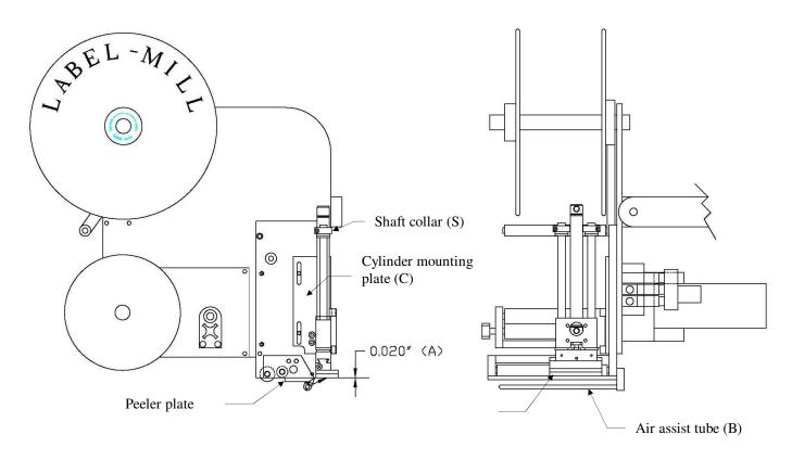
Tamp pad to peeler plate clearance and maximum cylinder travel
