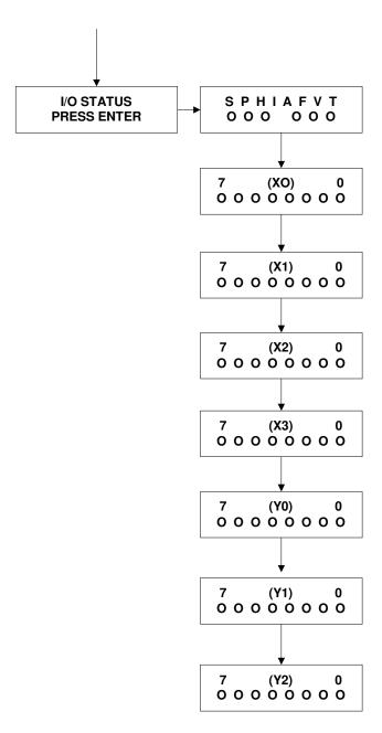
I/O Ports are numbered as follows 7 6 5 4 3 2 1 0 Ports are numbered from right to left.
