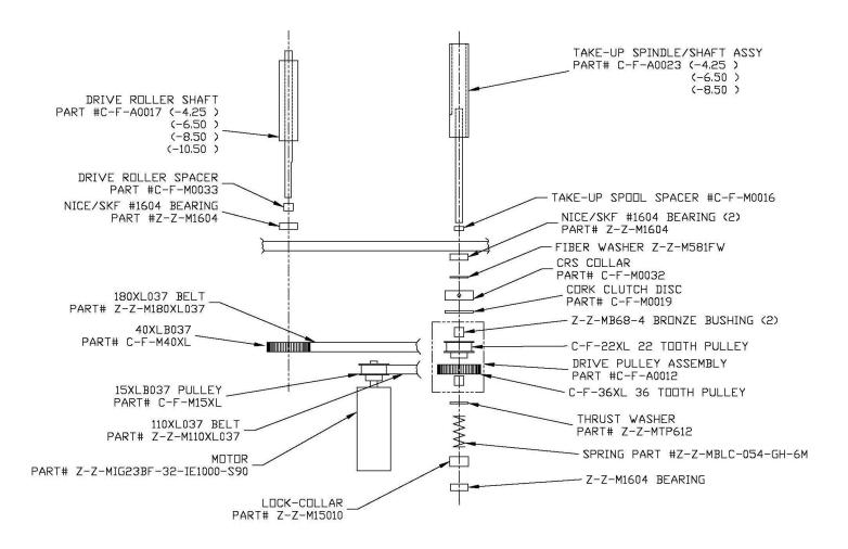
To reduce waste web tension, move the lock collar 1/32" away from the take-up spool. To increase waste web tension, move the lock collar 1/32" toward the take-up spool.
