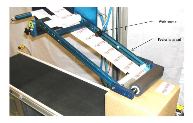
Manual adjustment of the label in relation to the peeler plate is achieved by loosening the thumbscrew on the backside of the web sensor and sliding the assembly up or down on the peeler arm rail.
