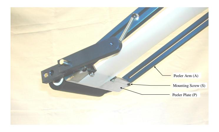
Peeler Plate Adjustment (used to adjust tracking)
