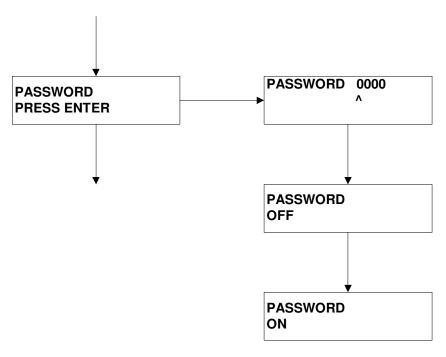
Note: use UP and DOWN arrows to toggle between "ON" and "OFF". The enter key will save selection.
