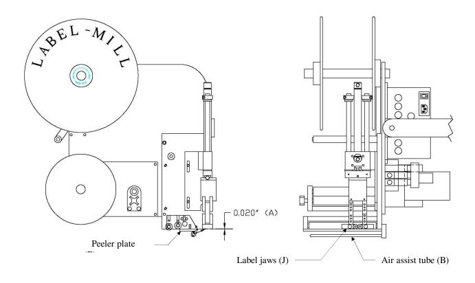
Label jaw to peeler plate clearance and maximum cylinder travel
