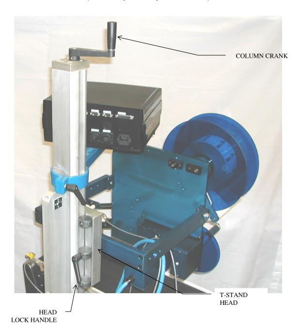
To adjust the T-150 mounting stand, simply loosen the headlocks and adjust to the desired height by turning the column crank. Be sure to lock the headlocks when finished.
